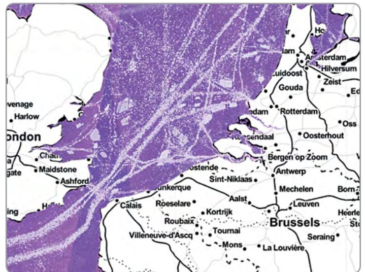
Maritime traffic in the Strait of Dover highlighted by a mosaic of all the Sentinel-1 images acquired in 2017.
