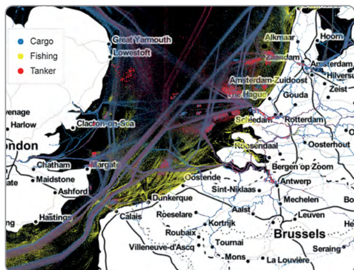
Distribution of AIS messages which are used to teach the system how to automatically recognize different ship types.
