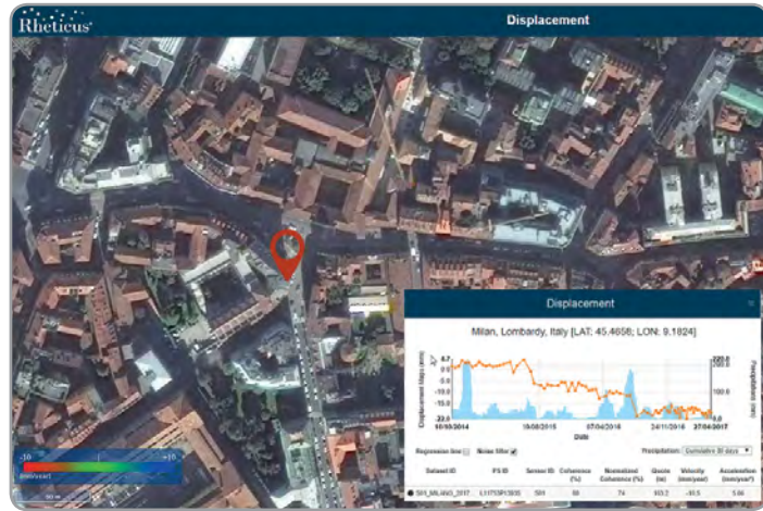
Milan, Italy. Screenshot of Rheticus® Displacement interface pinpointing where leaks are most likely and showing ground movements' velocity acceleration and trends.
