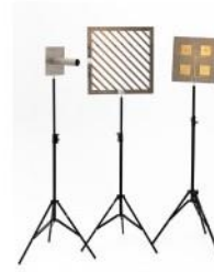
RADIO TRANSPARENCY AND TRANSMISSION MEASURING STAND
